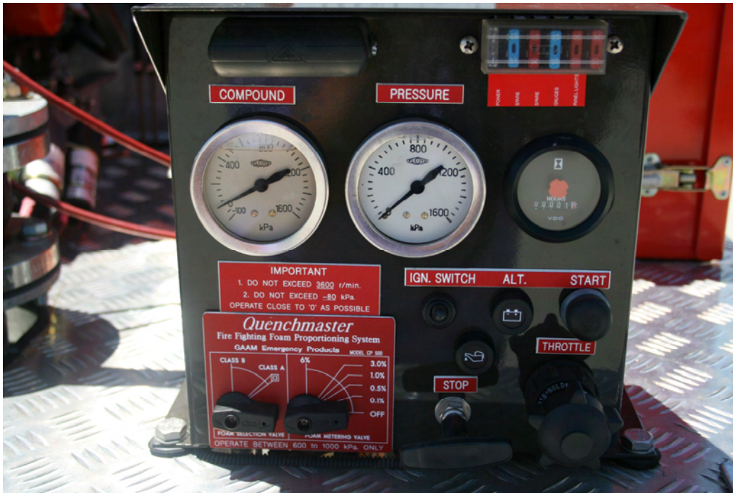
A typical Cat 7 Tanker pump control panel
